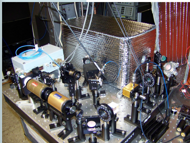
Adam's setup. The gray box at the left is the laser and the silver box at the back is the temperature controlled box. The optical cavity is in a vacuum chamber inside this box.
